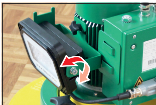
Fig. 10 The work light can be swiveled up and down.
