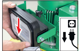
Fig. 3 Move the work light downwards.
