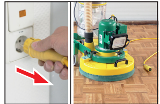
Fig. 9 Disconnect the power plug from the socket. → The work light goes off.
