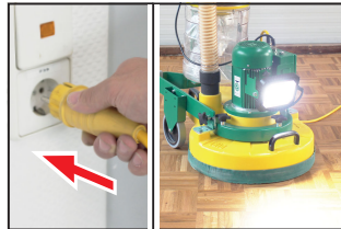
Fig. 8 Insert the mains plug into the socket. → The work light lights up.
